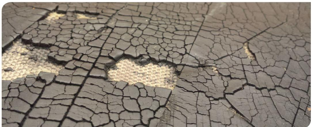
**Right:** Ozone cracking accelerates heat damage.
