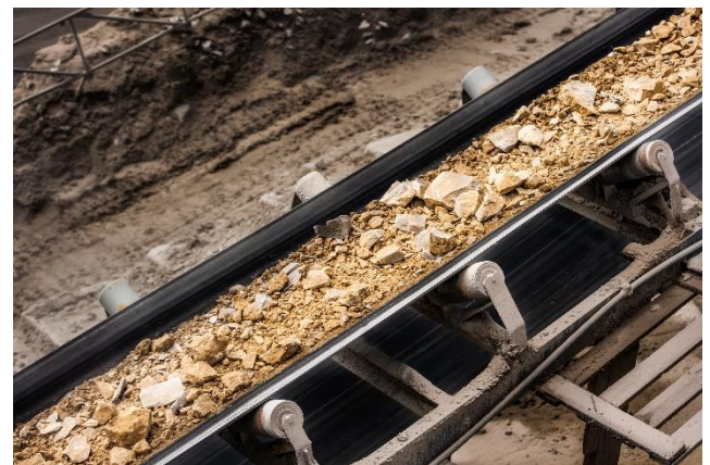
Above: Steelcord belt with breaker ply. Below: Steel cord belt in operation
