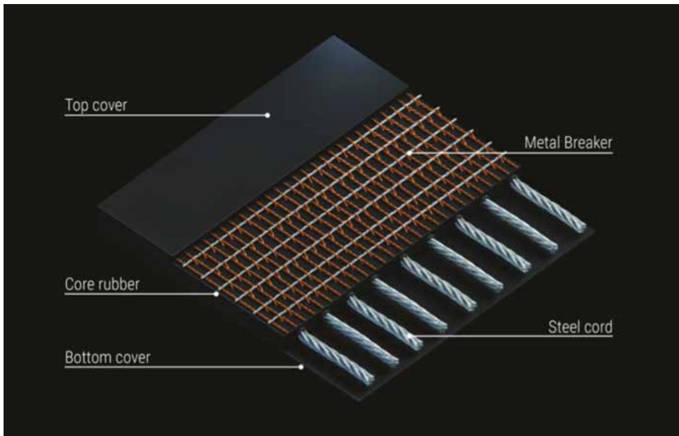
According to ISO 15236-1, a breaker ply should be positioned at a distance of between 1mm and 3mm from the longitudinal cords. The width of the breaker ply should be at least 10mm from the belt edge but no more than 100mm less than the width of the belt. On this basis the breaker ply is regarded as part of the cover, which means that the cover thickness is measured from the cords.
