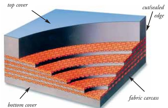
carcass, which typically contain layers of extremely strong but flexible fabric embedded in the rubber. It is the carcass that provides the inherent characteristics of a conveyor belt such as its tensile strength and elongation (elasticity or 'stretch' under tension).
