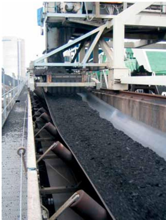
Wear on the bottom cover of the belt is mainly caused by the friction contact with the drum surface and idlers. The rate and uniformity of this type of wear can be adversely affected by many other factors such as misaligned or worn drums and idlers set at incorrect angles. Factors such as ozone penetration or an unclean environment where there is a build up of waste material can accelerate wear. Belt cleaning systems, especially steel edged scrapers, can also cause wear to the top cover surface.
