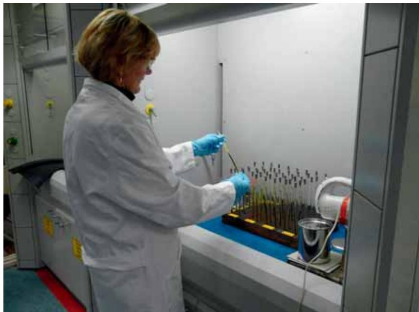
international standards using an ozone testing cabinet some years ago and by using special additives in its rubber compounds, it has ensured that every Dunlop belt exceeds international standards by a considerable margin.
