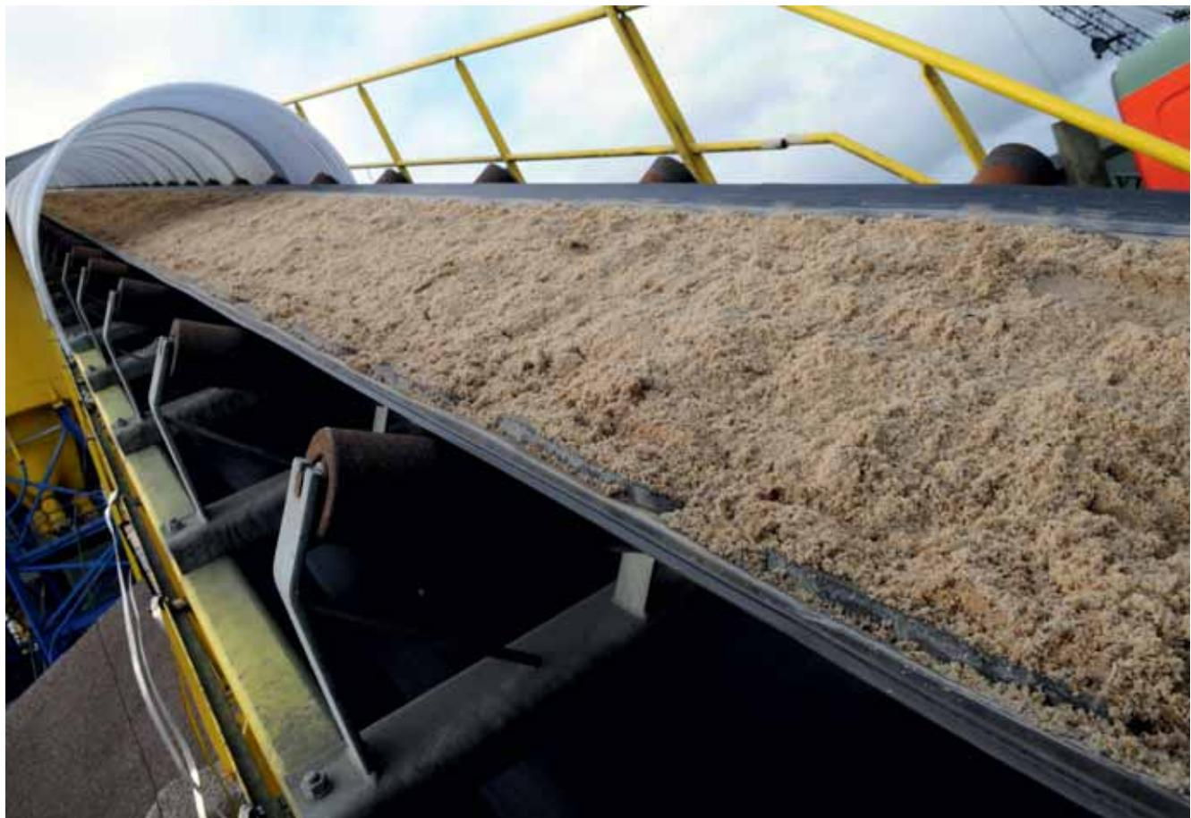
wear caused by abrasion (the most commonly used type), tearing and cutting, heat, fire and oil penetration. These different covers are generally referred to as 'cover grade qualities'.
