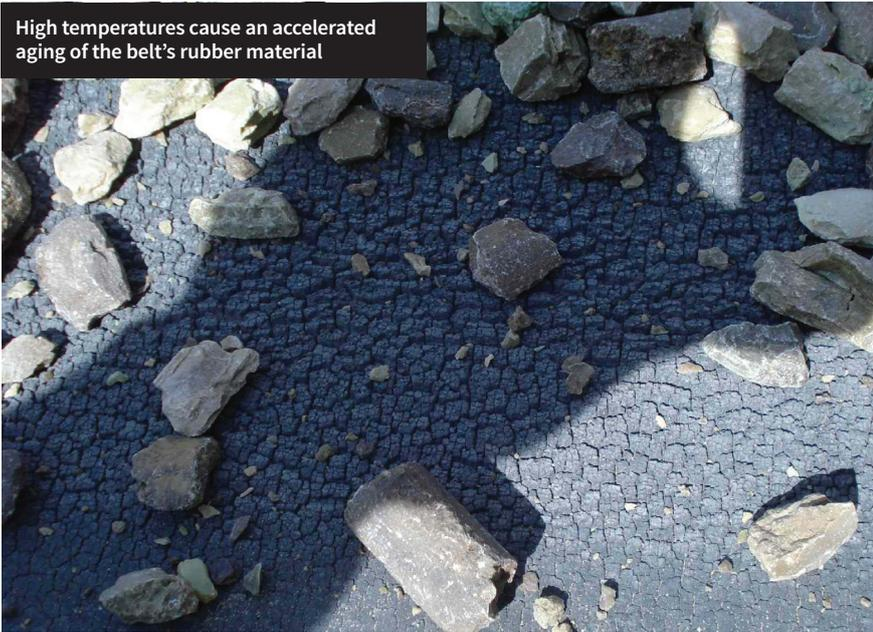
temperature of the conveyed material and the maximum temporary peak temperature. The two main classifications of heat resistance recognised in the market are T150, which relates to a maximum continuous temperature of 150 °C, and T200, which is for more extreme heat conditions up to 200 °C. Success or failure will depend on having accurate temperature data to give to potential belt suppliers.
