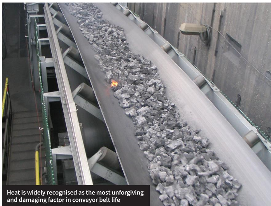
Heat is widely recognised as the most unforgiving and damaging factor in conveyor belt life
