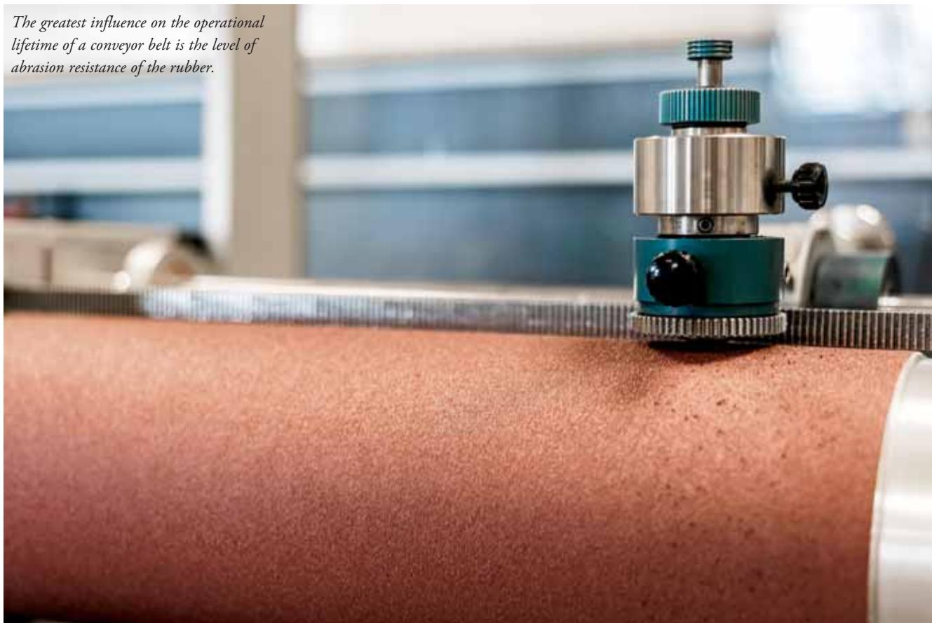
polyester/nylon (EP) fabric reinforced carcass protected by an outer cover of rubber. It is the carcass that provides the inherent characteristics of a conveyor belt such as its tensile strength and elongation (elasticity or 'stretch' under tension).
