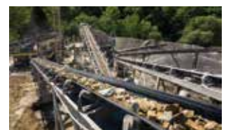
Ripping, tearing and impact – the best solution is to fit a conveyor belt specifically engineered for the purpose.
