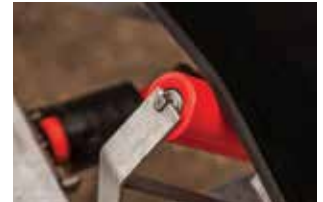
Belts that are too thick can cause problems such as excessive rigidity
