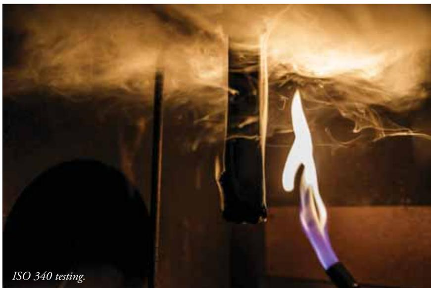
ISO 340 test with the covers intact on the belt samples whereas Class 2B requires that the belt is also able to pass the test with the top and bottom cover rubber removed. Both Class 2A and 2B fulfill the anti-static requirements of ISO 284.
