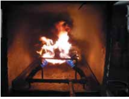
Class 4A entails EN12881-1 method A, C or D in addition to EN/ISO 340 testing.
