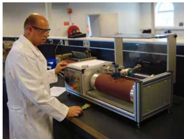
ISO 4649 / DIN 53516 abrasion testing.
