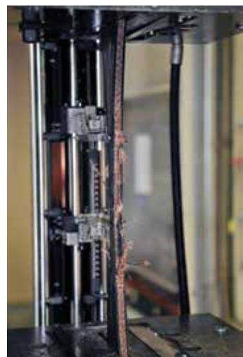
The tensile strength of a belt is measured according to the ISO 283 test method.
