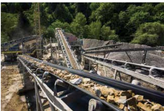
The use of EE fabrics instead of EP reduces troughability, impact resistance and rip resistance.
