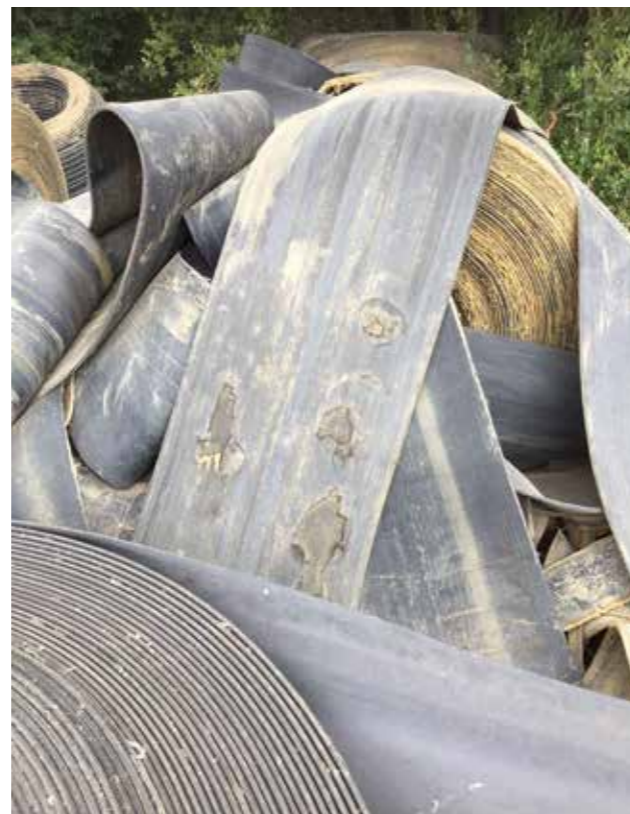
The use of imported 'sacrificial' belts is a never-ending 'fit, repair, replace' cycle.
