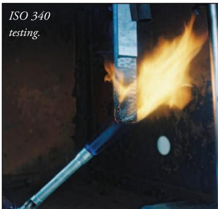
exposing six individual samples of belt to a naked flame causing them to burn. The source of the flame is then removed and the combustion time (duration of flame) of the test piece is recorded. A current of air is then applied to the test piece for a specified time after the removal of the flame. The flame should not re-ignite.
